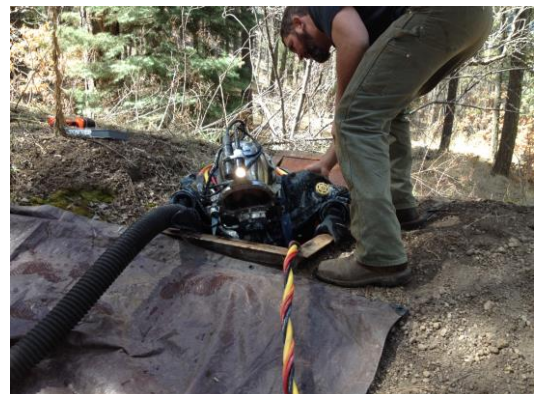
Figure 11. Squeezing skinniest diver into Tank 2's 18 1/2 x 24 inch hatch in System 2.
