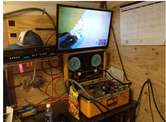
Figure 10. A special blue food dye solution is used to detect leaks in any locations below the water in the tanks. Obviously, the dye would go into a tank puncture and not just float by the potential puncture as seen here. Several of the System 1 tanks did have roots penetrating the tank sidewalls.
